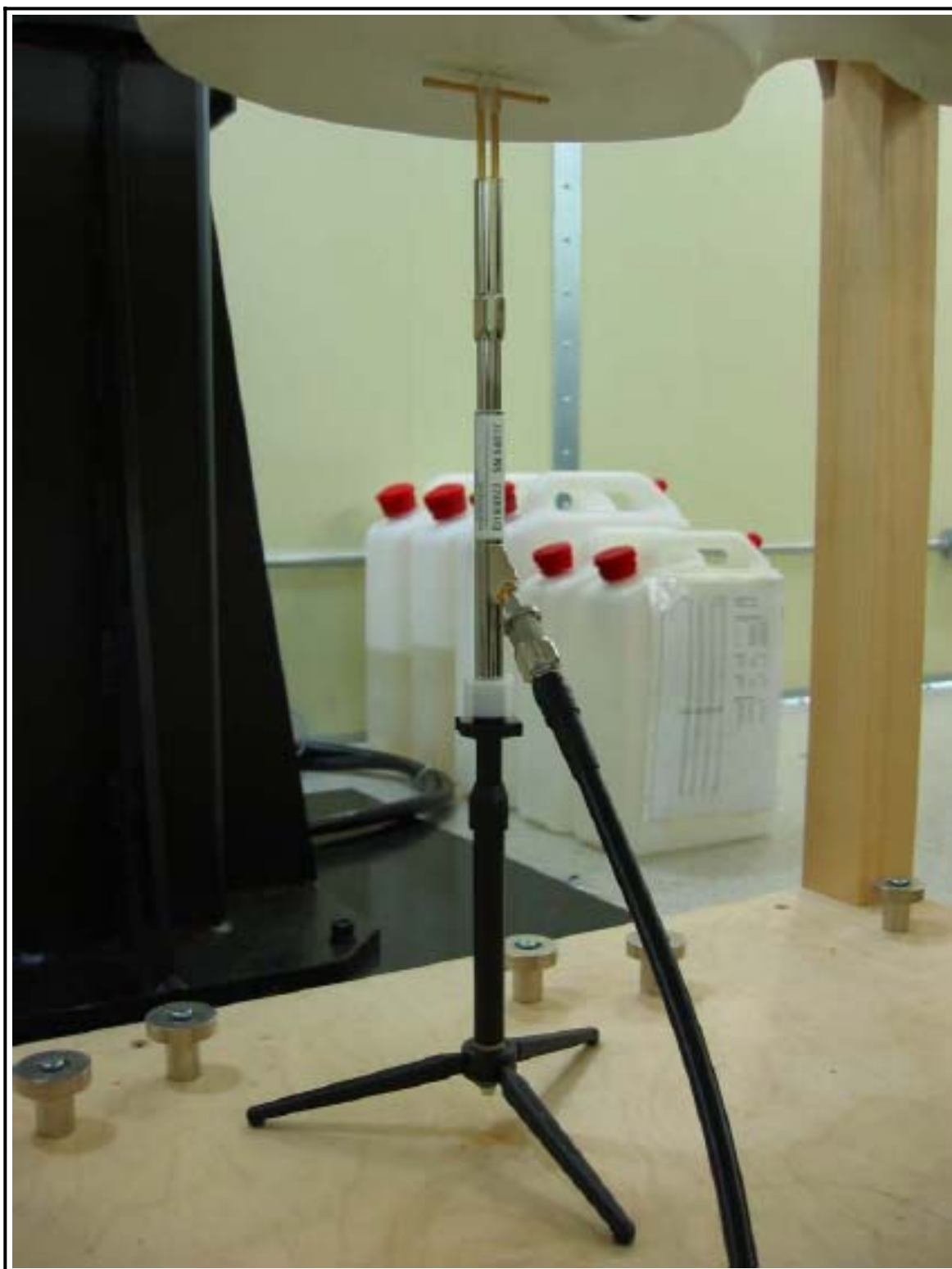
Figure 2 1900 MHz Dipole Validation Test Setup
