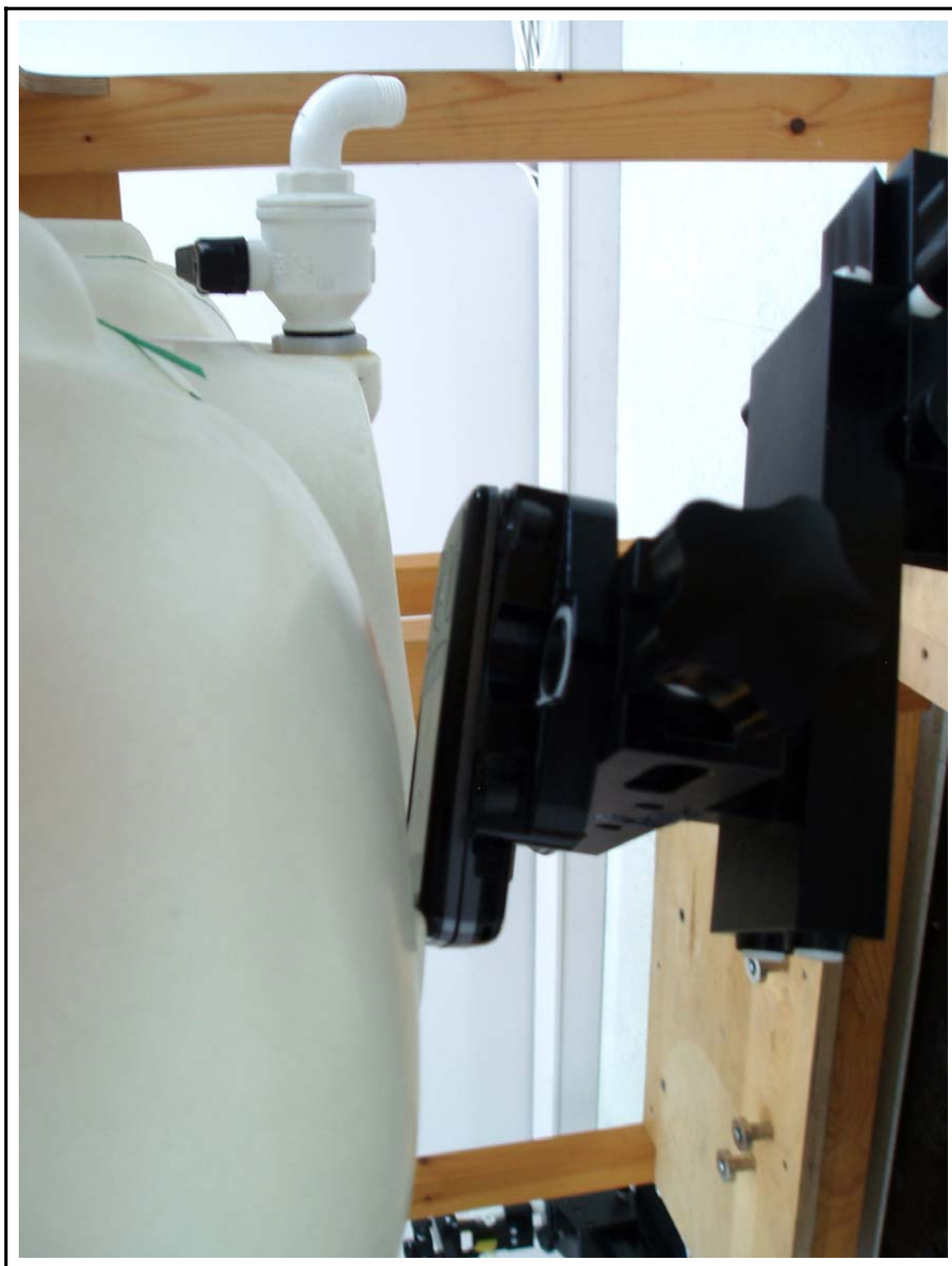
Figure 3 Right Head SAR Test Setup - Ear Tilt Position
