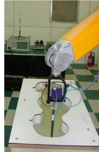
Figure 3.2 Photograph of the probe and the Phantom
