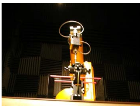
Figure 3-1 HAC RF Emissions Measurement System
