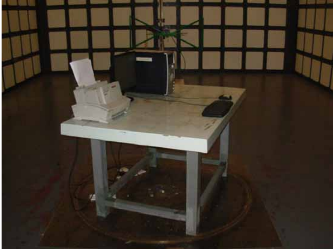
SETUP WITH MAXIMUM DETECTED EMISSION AT HORIZONTAL POLARIZATION (M/N: L1742SEU, TEST MODE: D-SUB 1280*1024@75Hz)
