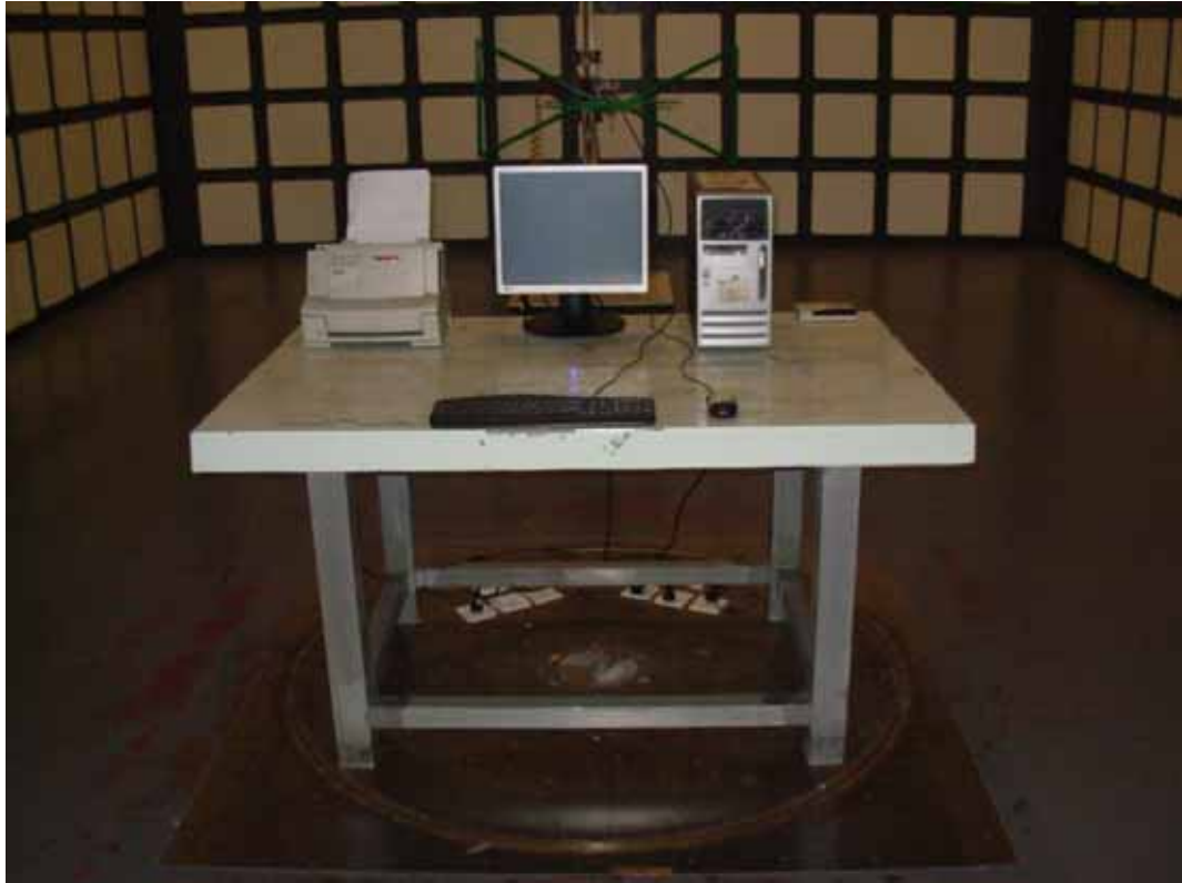
FRONT VIEW OF RADIATED EMISSION TEST
