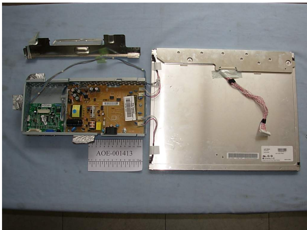
FIGURE 5 LCD MONITOR (M/N: L1753HMS) MAIN BOARD (COMPONENT SIDE)
