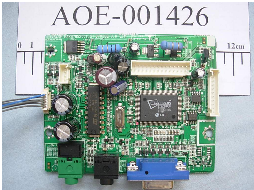
FIGURE 8 LCD MONITOR (M/N: L1754SMS) MAIN BOARD (COMPONENT SIDE)
