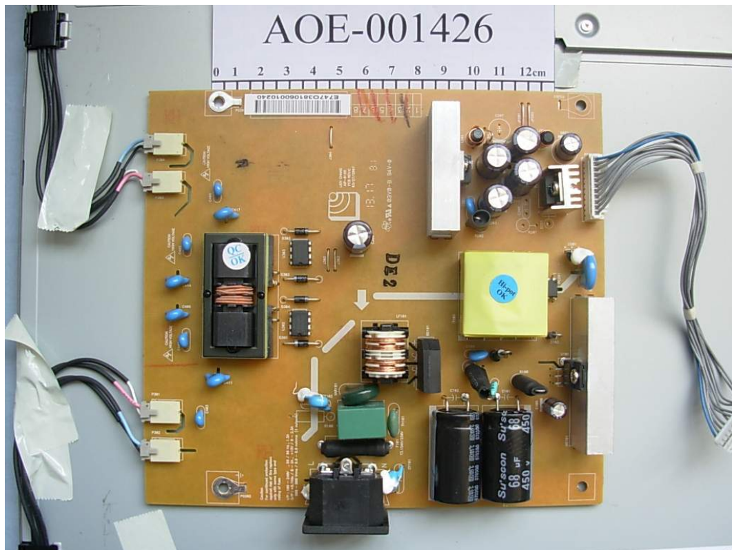
FIGURE 12 LCD MONITOR (M/N: L1754SMS) POWER BOARD (SOLDERED SIDE)
