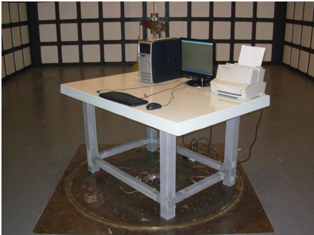
SETUP WITH MAXIMUM DETECTED EMISSION AT VERTICAL POLARIZATION (VGA 1280*1024@60Hz, Low FREQUENCY)
