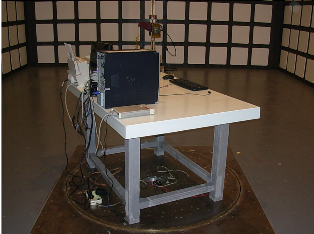
SETUP WITH MAXIMUM DETECTED EMISSION AT HORIZONTAL POLARIZATION (VGA 1280*1024@60Hz, Low FREQUENCY)
