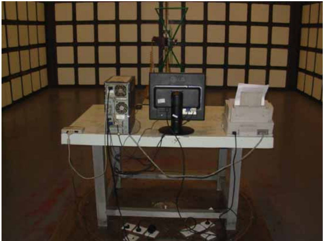
BACK VIEW OF RADIATED EMISSION TEST
