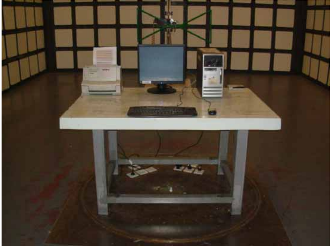
FRONT VIEW OF RADIATED EMISSION TEST
