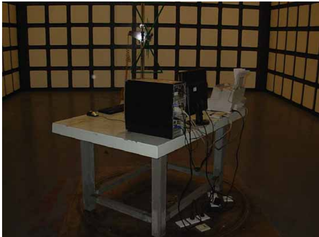
SETUP WITH MAXIMUM DETECTED EMISSION AT VERTICAL POLARIZATION (TEST MODE: D-SUB 1280*1024@75Hz)
