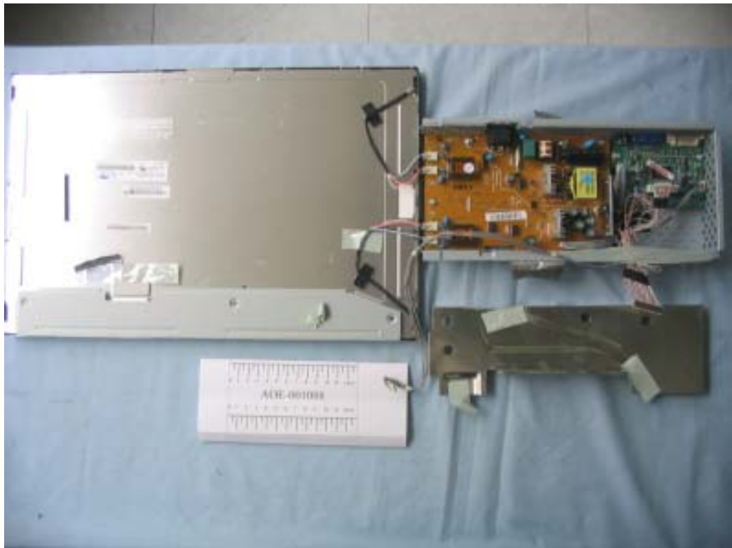
FIGURE 7 LCD MONITOR (M/N: L194WTM) MAIN BOARD REMOVED
