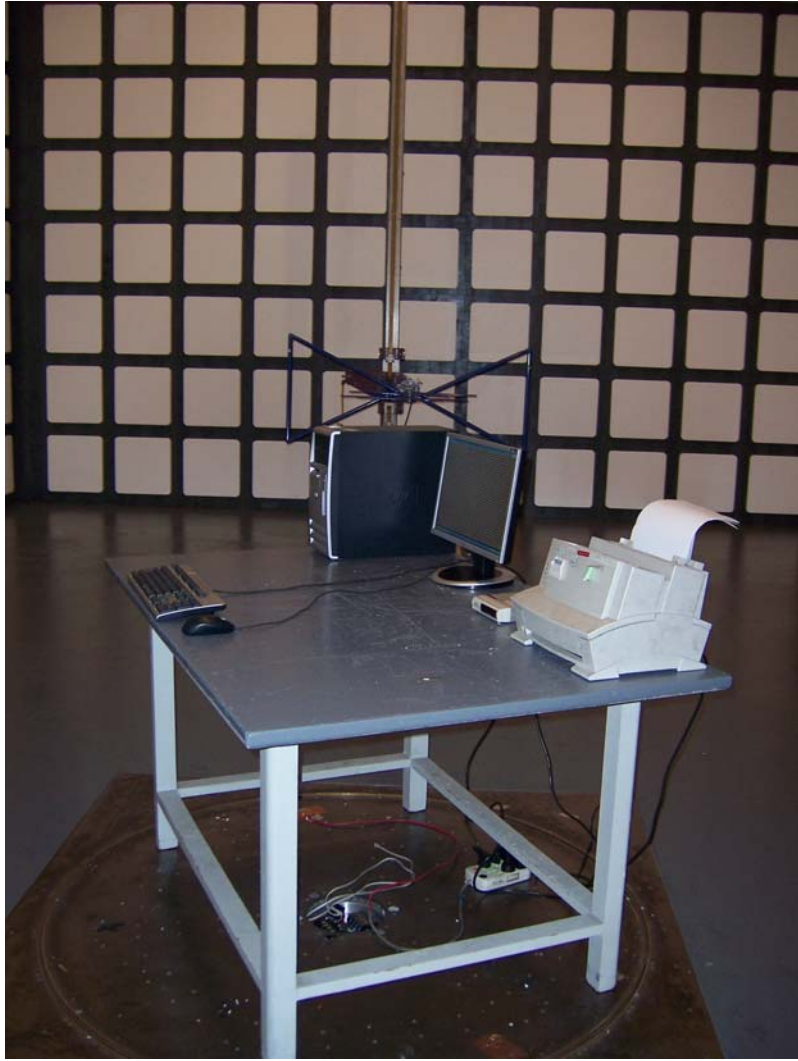
SETUP WITH MAXIMUM DETECTED EMISSION AT HORIZONTAL POLARIZATION (DVI 1280*1024@75Hz)
