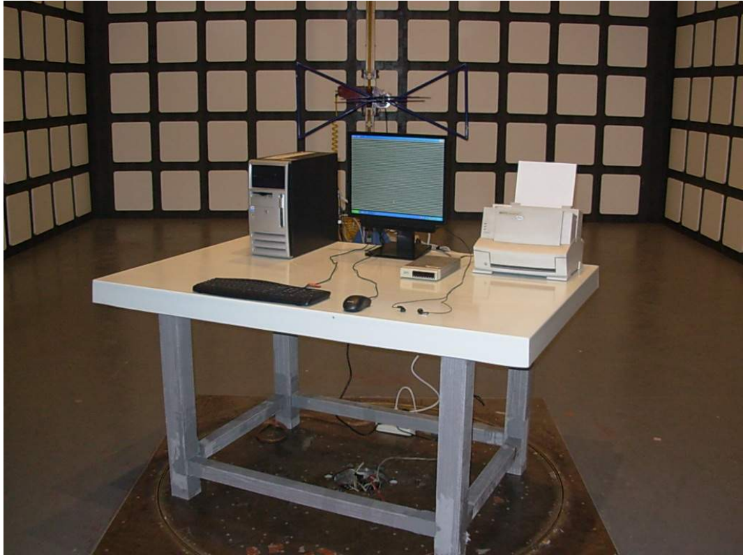
SETUP WITH MAXIMUM DETECTED EMISSION AT HORIZONTAL POLARIZATION (DVI 1024*768@60Hz)
