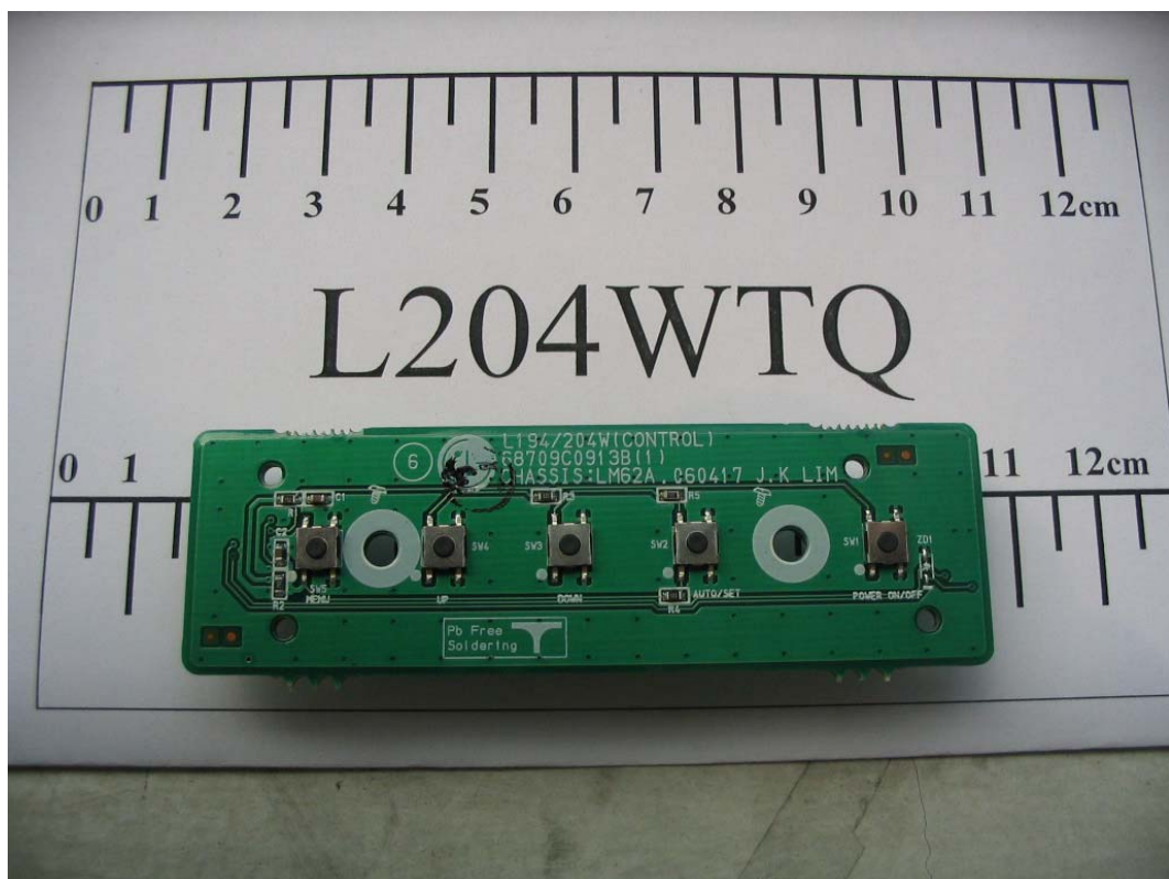
FIGURE 3 LCD MONITOR (M/N: L204WTQ) CONTROL BOARD (SOLDERED SIDE)
