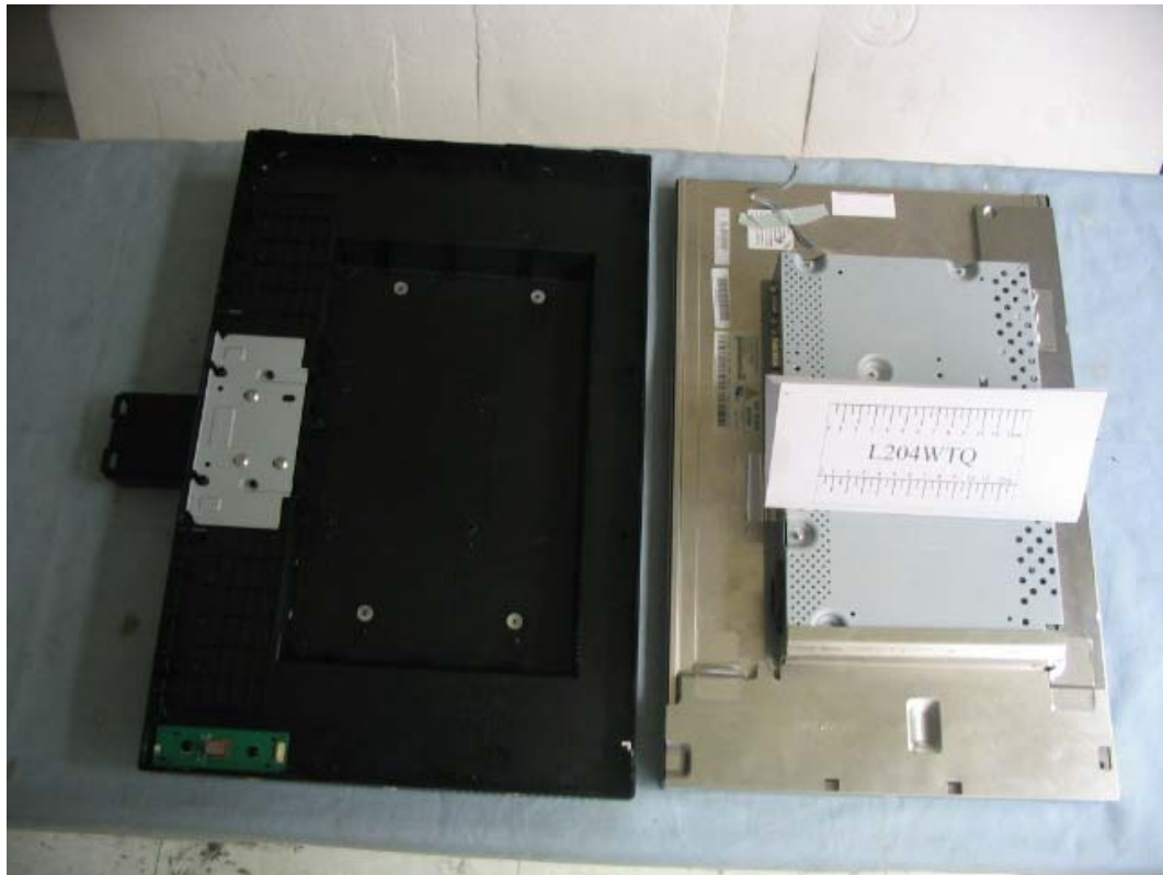
FIGURE 1 LCD MONITOR (M/N: L204WTQ) BACK SHELL REMOVED
