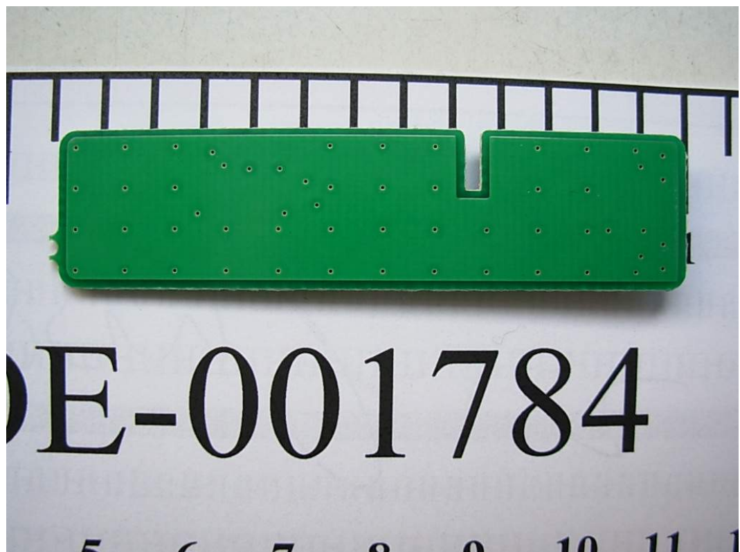
FIGURE 5 LCD MONITOR (M/N: L226WUQS) LED BOARD (SOLDERED SIDE)
