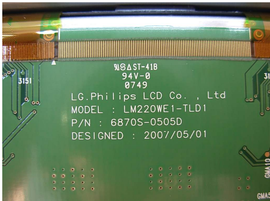
FIGURE 21 LCD MONITOR (M/N: L226WUQS) LCD PANEL MAIN BOARD LABEL
