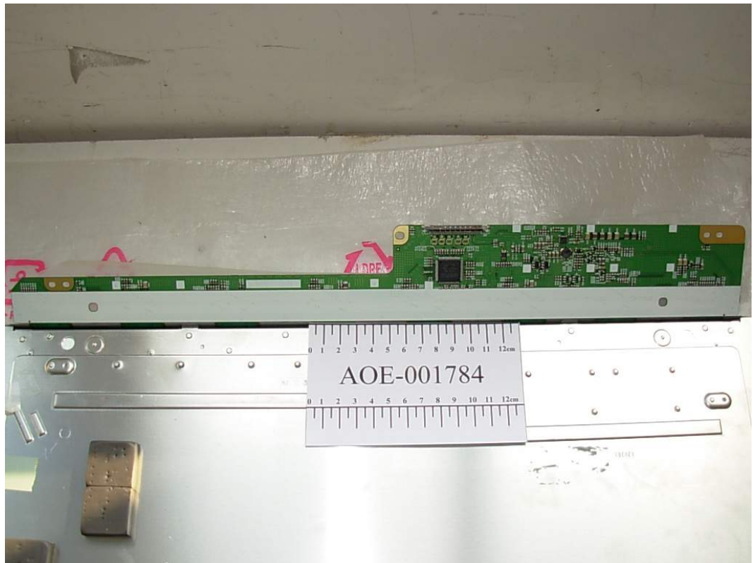
FIGURE 18 LCD MONITOR (M/N: L226WUQS) LCD PANEL MAIN BOARD (COMPONENT SIDE)
