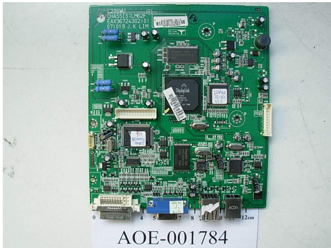
FIGURE 7 LCD MONITOR (M/N: L226WUQS) MAIN BOARD (COMPONENT SIDE)
