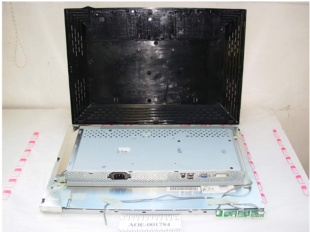
FIGURE 1 LCD MONITOR (M/N: L226WUQS) COVER REMOVED
