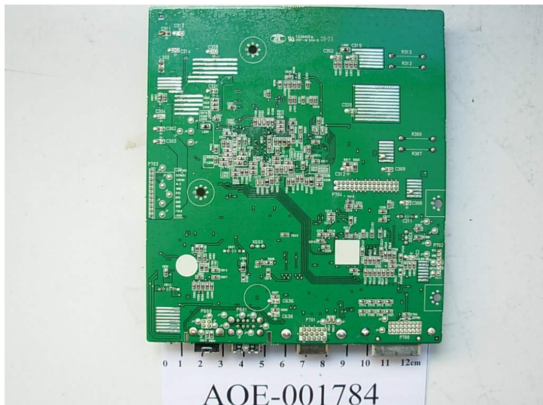
FIGURE 8 LCD MONITOR (M/N: L226WUQS) MAIN BOARD (SOLDERED SIDE)
