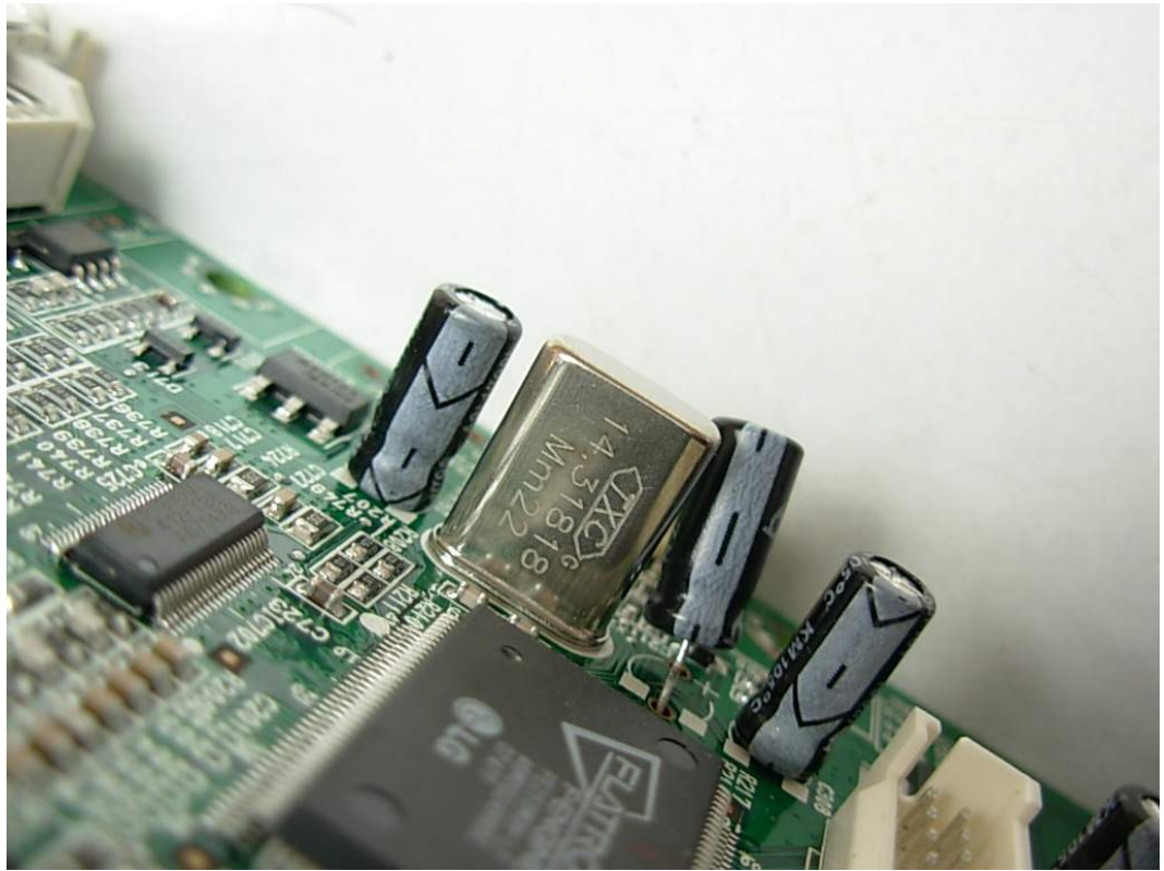
FIGURE 9 LCD MONITOR (M/N: L226WUQS) CRYSTAL #1 ON MAIN BOARD
