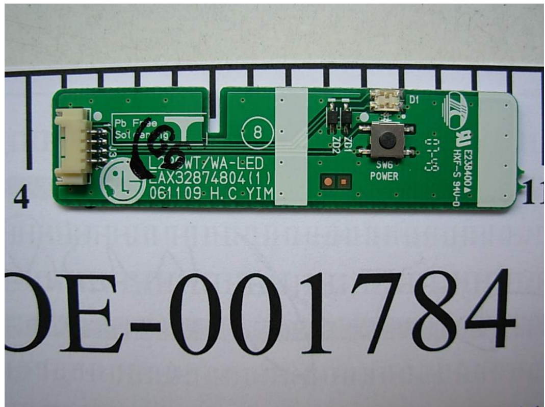
FIGURE 4 LCD MONITOR (M/N: L226WUQS) LED BOARD (COMPONENT SIDE)
