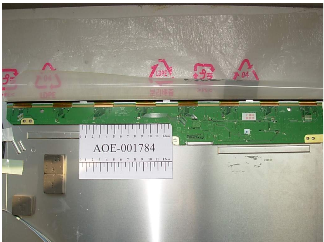
FIGURE 19 LCD MONITOR (M/N: L226WUQS) LCD PANEL MAIN BOARD (SOLDERED SIDE)
