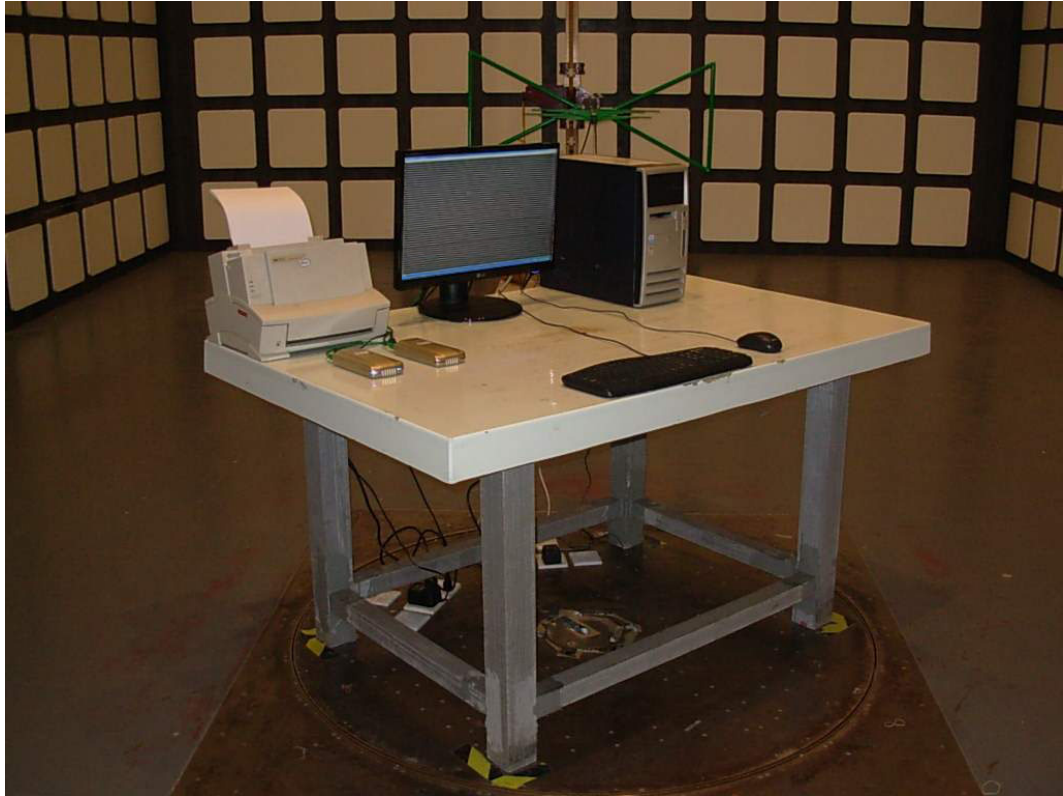
SETUP WITH MAXIMUM DETECTED EMISSION AT HORIZONTAL POLARIZATION (DVI 1680*1050@60Hz & USB CONNECTING)
