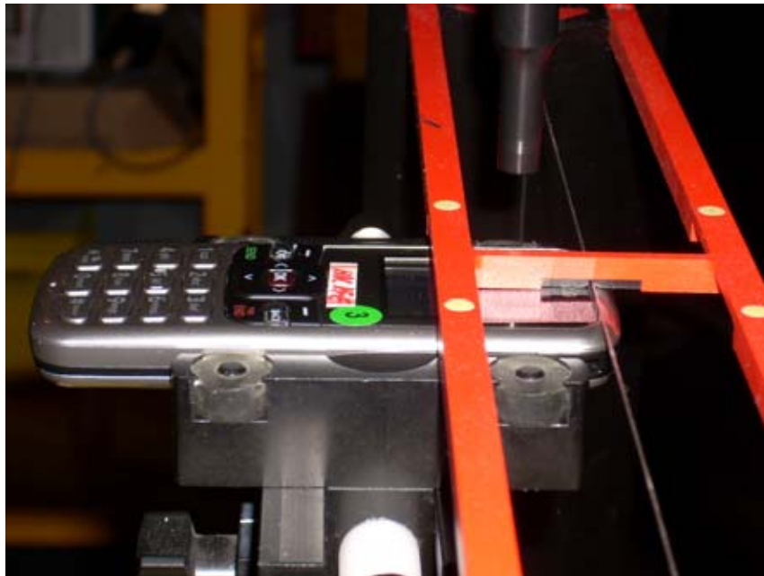
Figure 17-1 Ear Reference Point HAC Phantom Alignment
