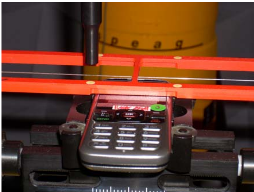
Figure 17-2 HAC Phantom Plane Alignment
