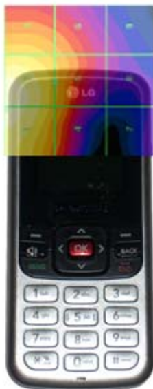
Figure 17-4 E-Field WD Scan overlay
