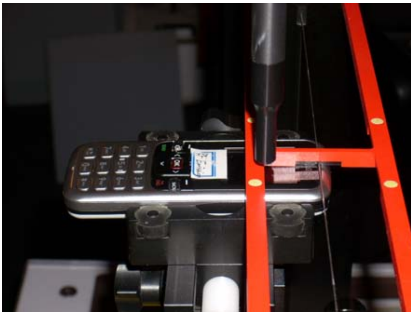
Figure 17-1 Ear Reference Point HAC Phantom Alignment
