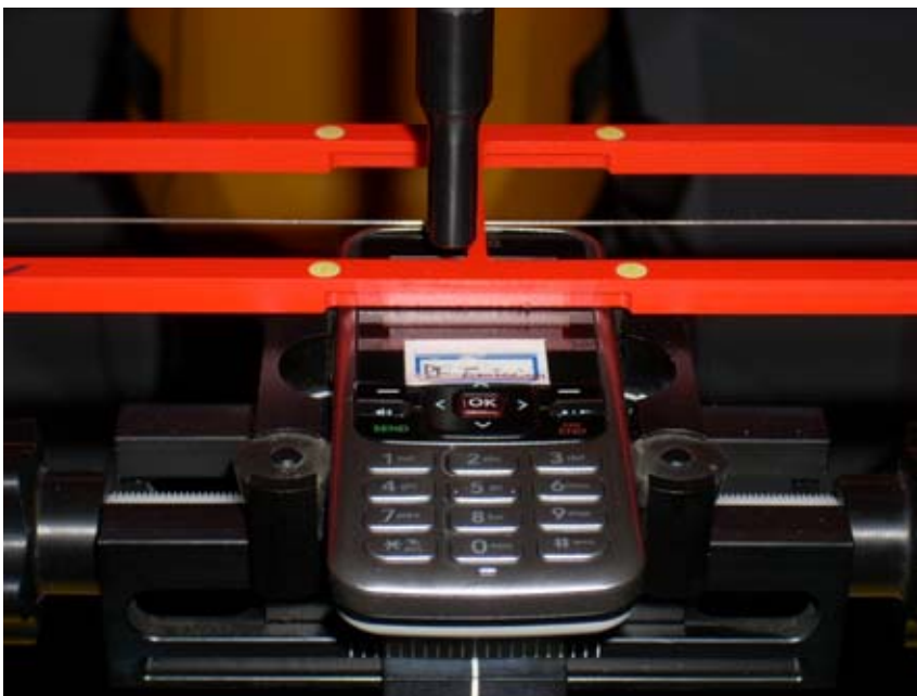
Figure 17-2 HAC Phantom Plane Alignment
