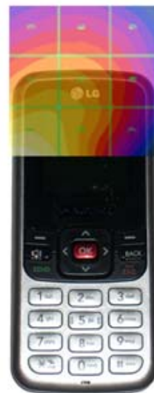
Figure 17-5 H-Field WD Scan overlay
