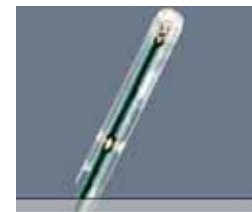
Figure 5-2 H-Field Free-space Probe
