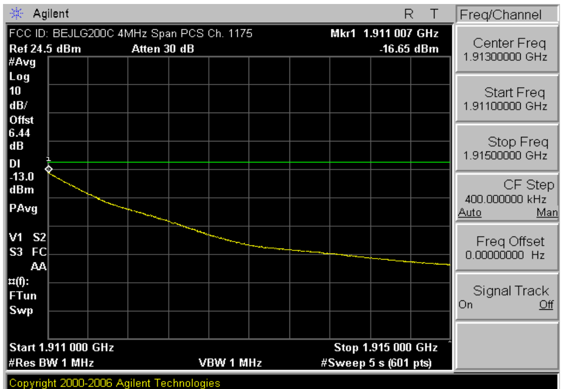
Plot 7-22. 4MHz Span Plot (PCS CDMA Mode – Ch. 1175)
