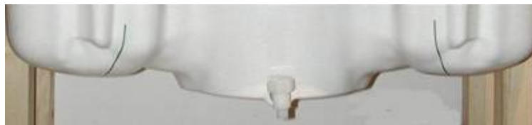
Figure 7-2 SAM Twin Phantom Shell
