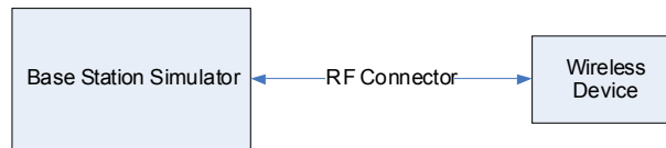
Figure 11-1 Power Measurement Setup
