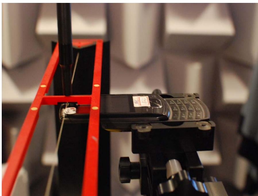
Figure 16-2 HAC Phantom Plane Alignment
