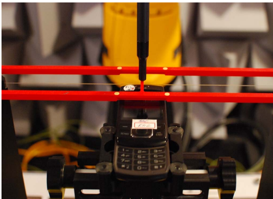
Figure 16-1 Ear Reference Point HAC Phantom Alignment
