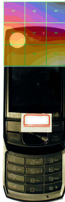
Figure 16-5 H-Field WD Scan overlay
