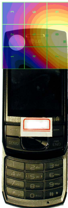
Figure 16-4 E-Field WD Scan overlay
