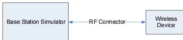
Figure 11-1 Power Measurement Setup
