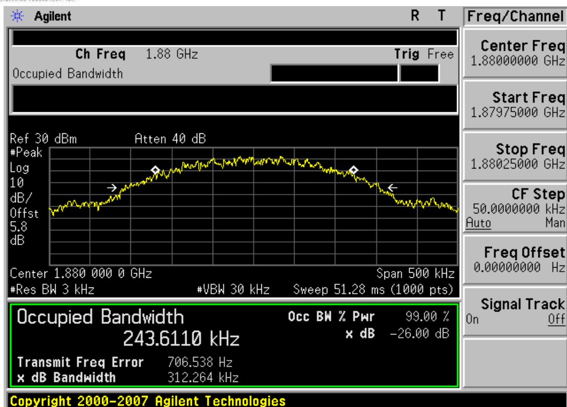
Plot 7-15. Occupied Bandwidth Plot (PCS GSM Mode – Ch. 661)
