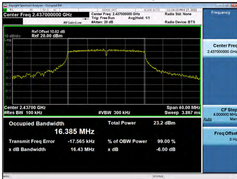
6 dB Bandwidth plot (802.11g-CH 6)
