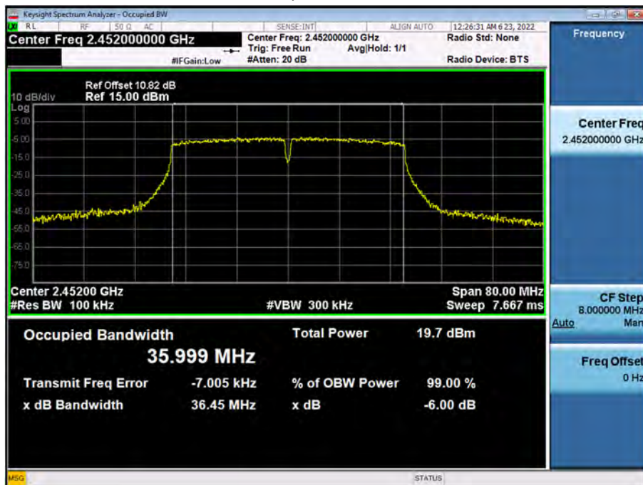
6 dB Bandwidth plot (802.11n_HT40-CH 9)
