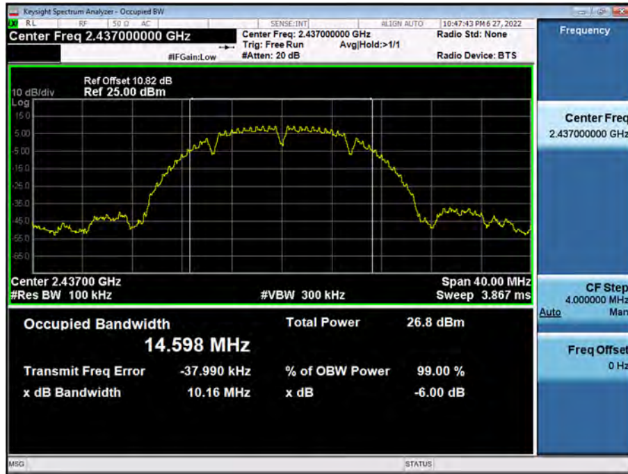
6 dB Bandwidth plot (802.11b-CH 6)
