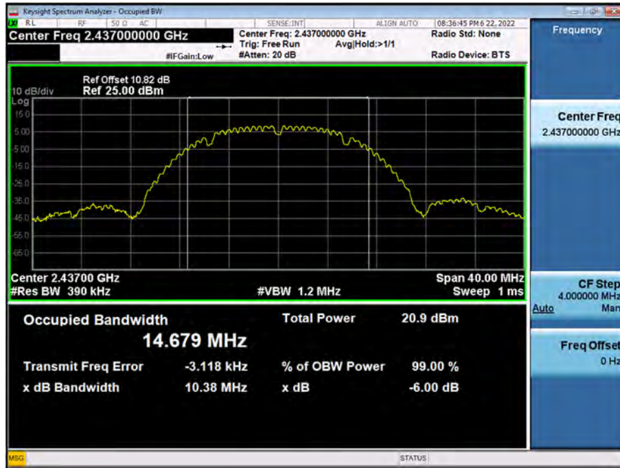
99% Bandwidth plot (802.11b-CH 6)
