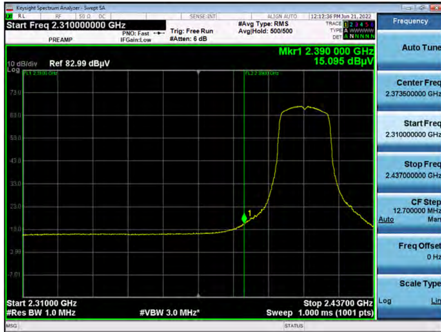
Radiated Restricted Band Edges plot – Peak Reading (802.11n Ch.01, Z-H)
