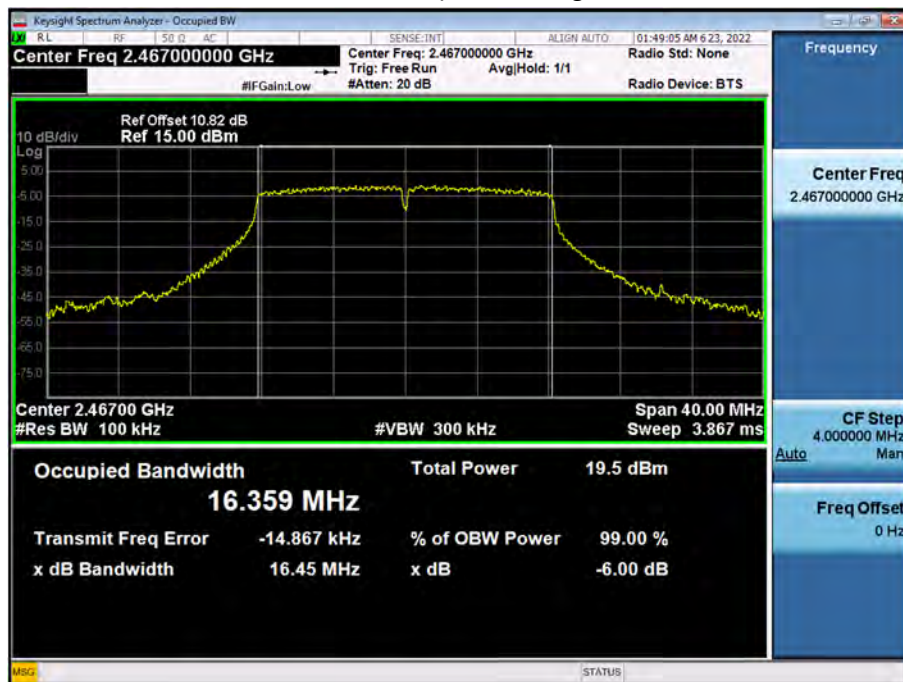
6 dB Bandwidth plot (802.11g-CH 12)
