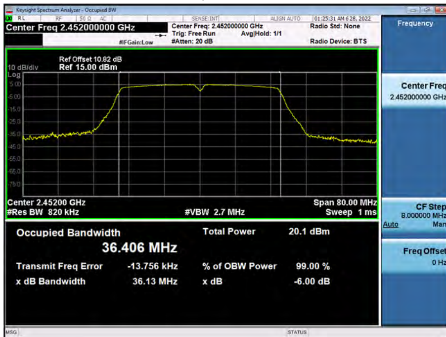
99% Bandwidth plot (802.11n_HT40-CH 9)
