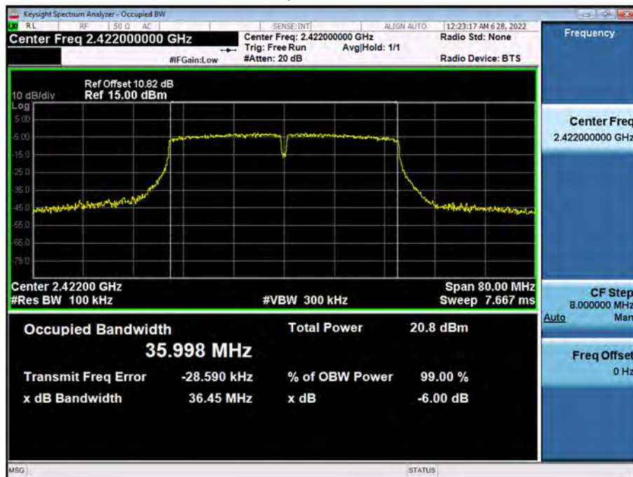
6 dB Bandwidth plot (802.11n_HT40-CH 3)
