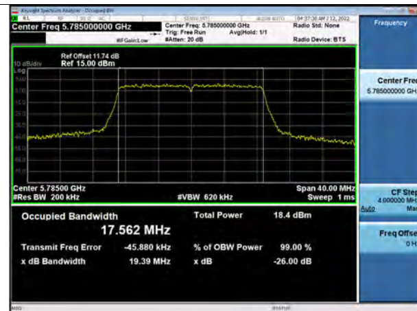
802.11ac_VHT20 UNII 3 BAND 26dB Bandwidth(CH 157)
