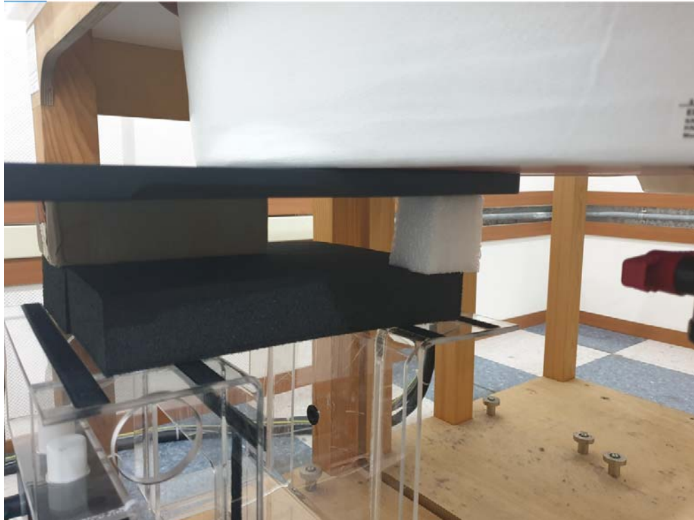
SAR Test Picture(Front)_Aux, Test separation distance : 0 mm
