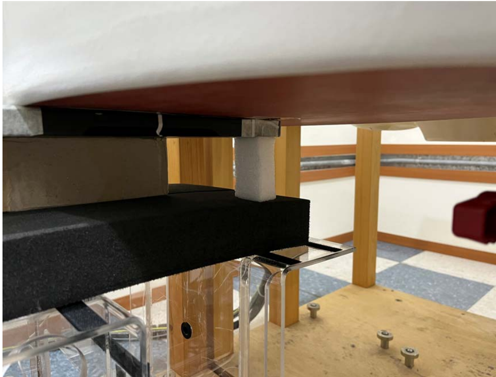
SAR Test Picture(Front)_Aux, Test separation distance : 0 mm
