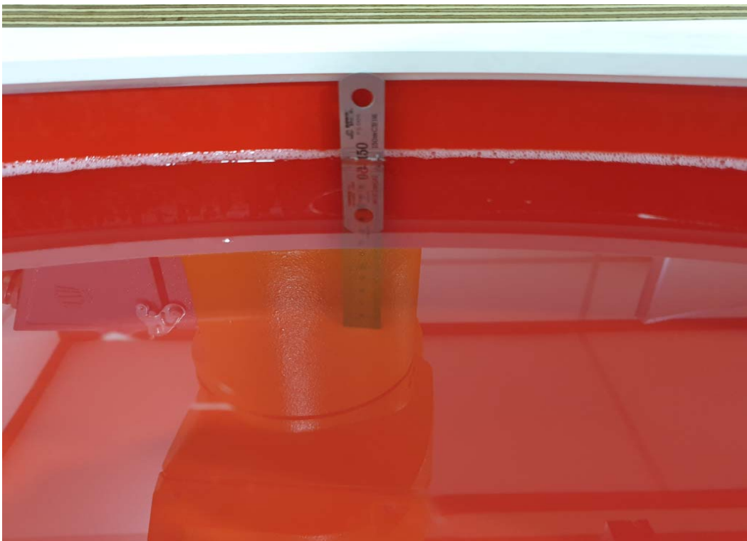
5 GHz (Head) Tissue Simulating Liquid, Depth: 150 mm
