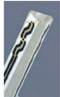
Figure E.2.2 Probe Thick-Film Technique
