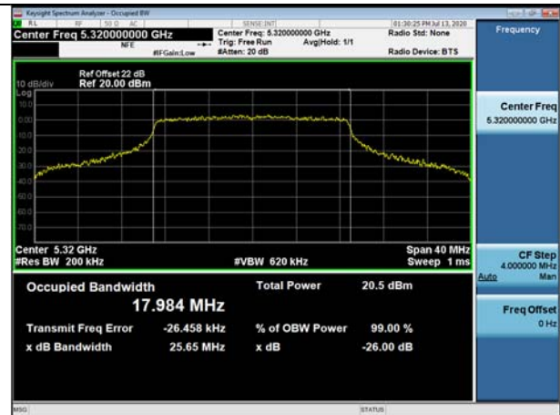
802.11n_HT20 UNII 3 BAND 26dB Bandwidth(CH 165)
