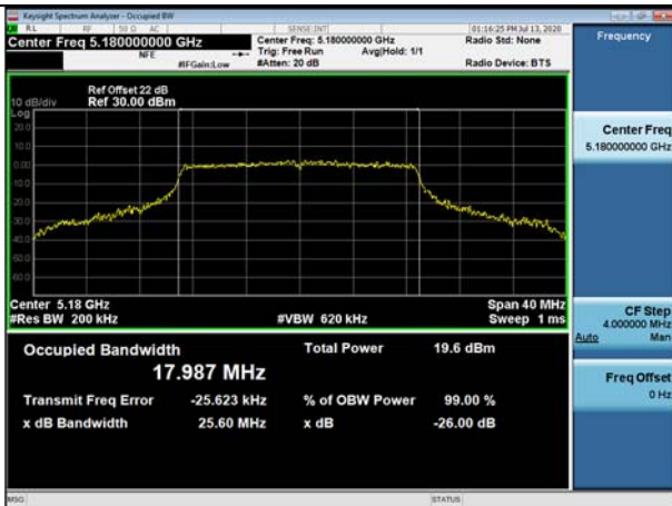
802.11n_HT20 UNII 2C BAND 26dB Bandwidth(CH 144)
