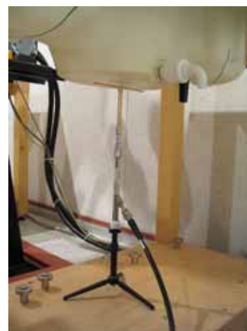
Photo of the dipole Antenna
