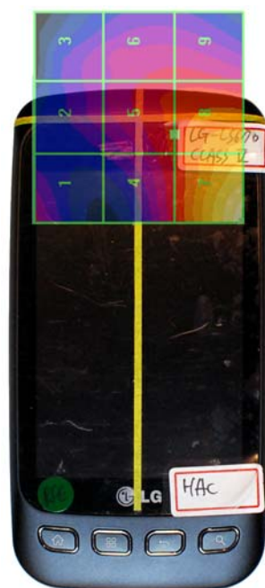
Figure 17-5 H-Field WD Scan overlay
