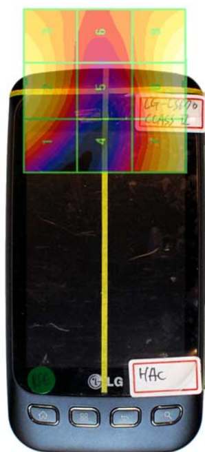
Figure 17-4 E-Field WD Scan overlay
