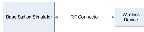
Figure 11-1 Power Measurement Setup
