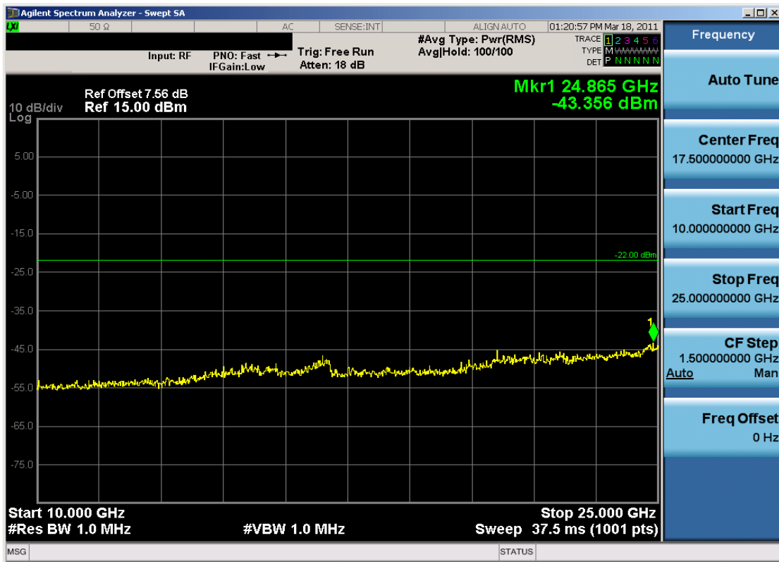
Plot 6-26. Conducted Spurious Plot (802.11b – Ch. 1)
