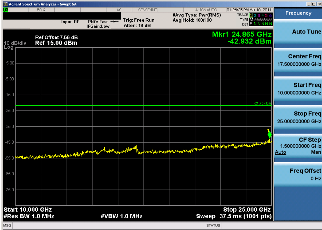
Plot 6-28. Conducted Spurious Plot (802.11b – Ch. 6)
