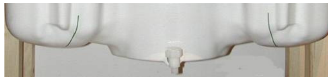
Figure 7-2 SAM Twin Phantom Shell
