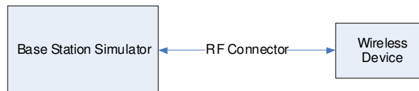
Figure 11-1 Power Measurement Setup
