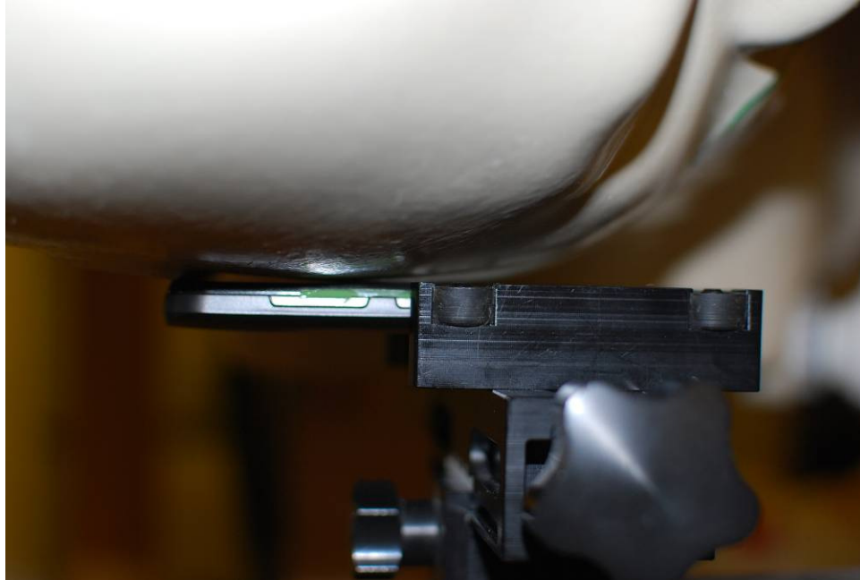
Figure 21-1 SAR Test Setup Photo 1 – Right Touch
