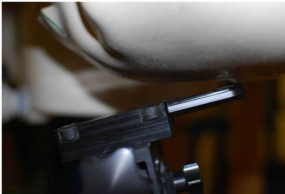
Figure 21-4 SAR Test Setup Photo 4 – Left Tilt
