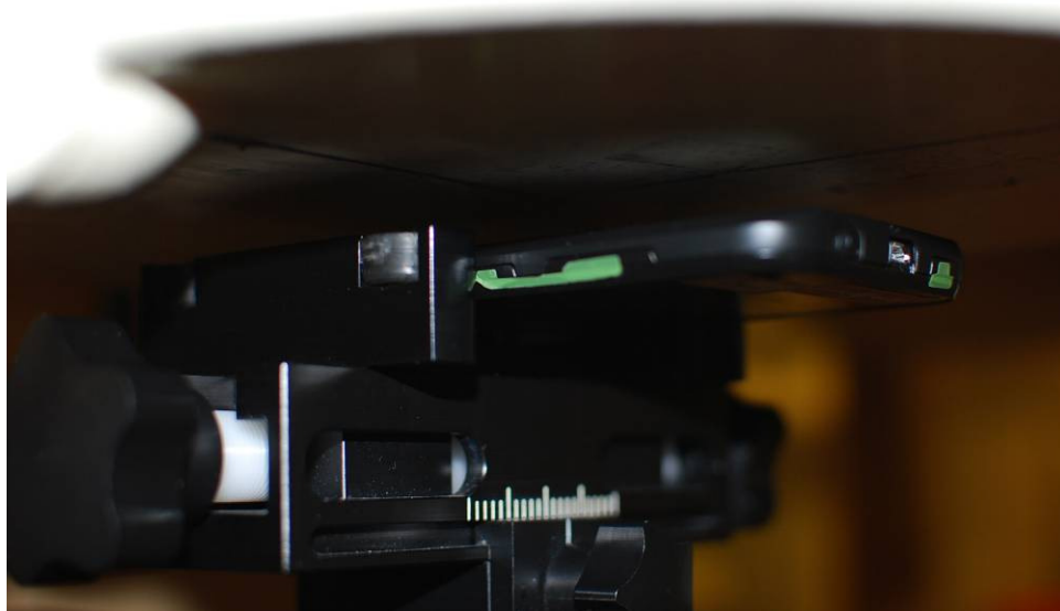
Figure 21-5 SAR Test Setup Photo 5 – Body Back at 1.0 cm
