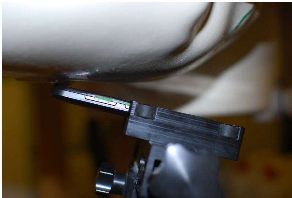
Figure 21-2 SAR Test Setup Photo 2 – Right Tilt
