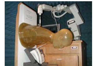
Fig. 1 SAR Test Setup
