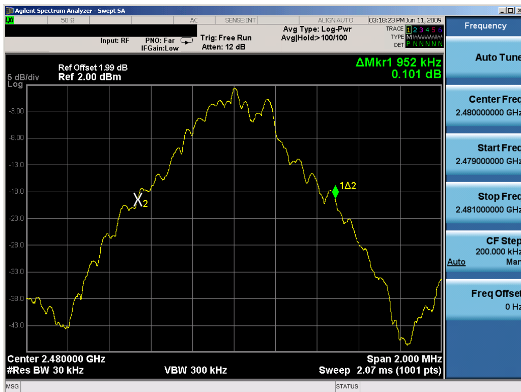
Plot 6-3. 20dB Bandwidth Plot (Bluetooth 1.0 – Ch. 78)
