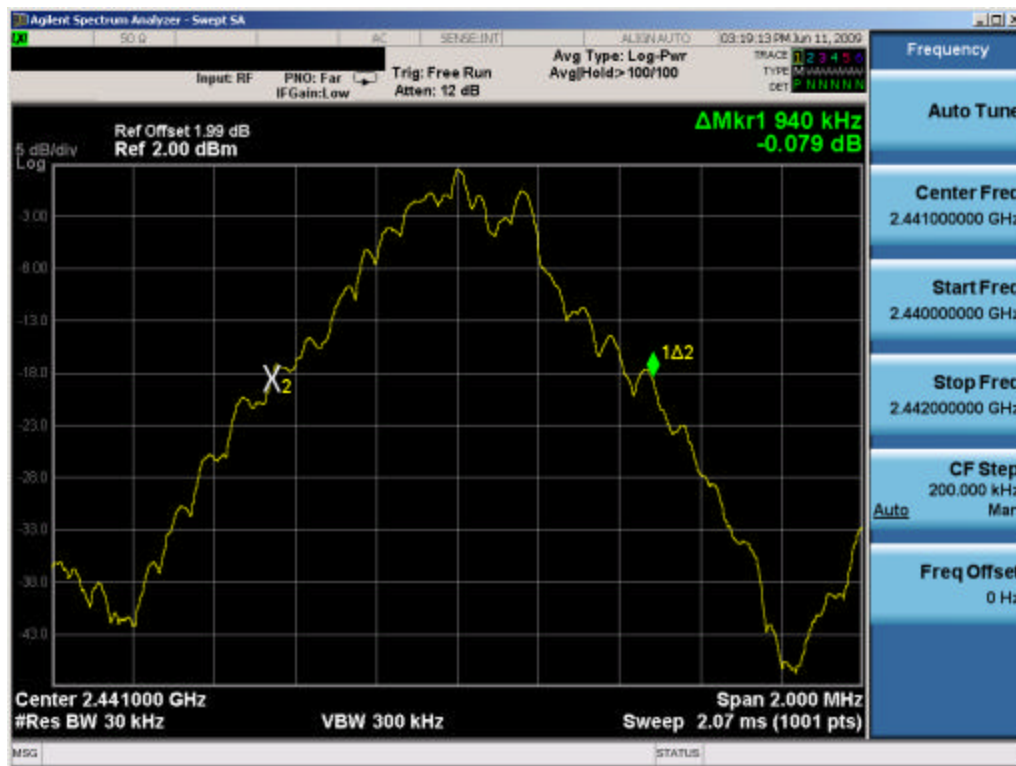
Plot 6-2. 20dB Bandwidth Plot (Bluetooth 1.0 – Ch. 39)
