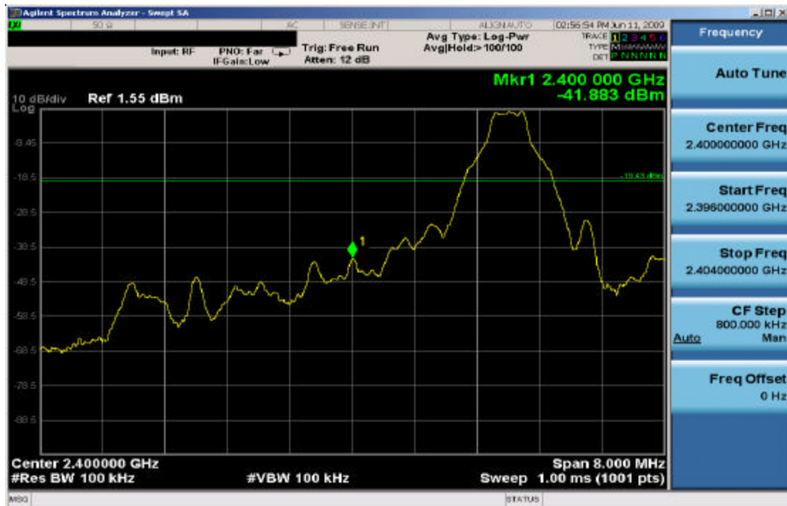
Plot 6-4. Band Edge Plot (Bluetooth – Ch. 0)
