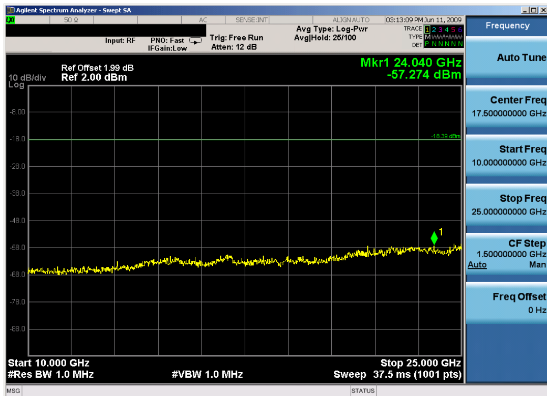
Plot 6-15. Conducted Spurious Plot (Bluetooth – Ch. 78)
