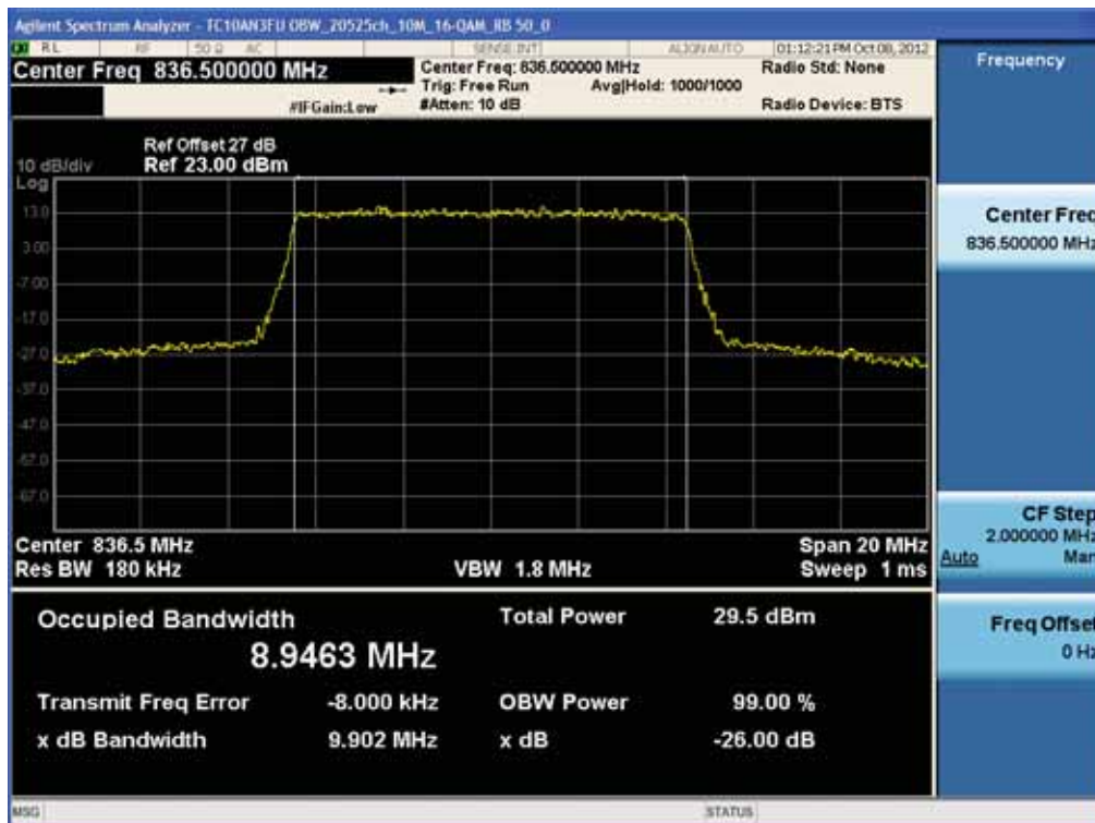
BAND 5. Occupied Bandwidth Plot (20525ch_10MHz_16-QAM_RB 50_0)
