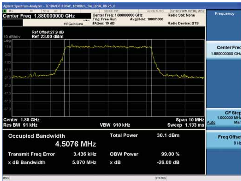
BAND 2. Occupied Bandwidth Plot (18900ch_5MHz_QPSK_RB 25_0)
