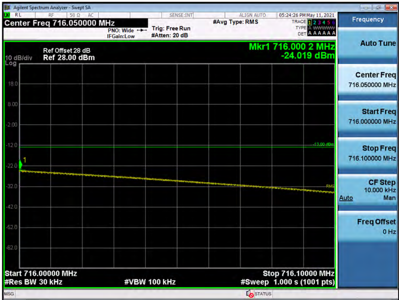
BAND 17. Upper Band Edge Plot (5M BW Ch.23825 QPSK_RB1_Offset 24)_1
