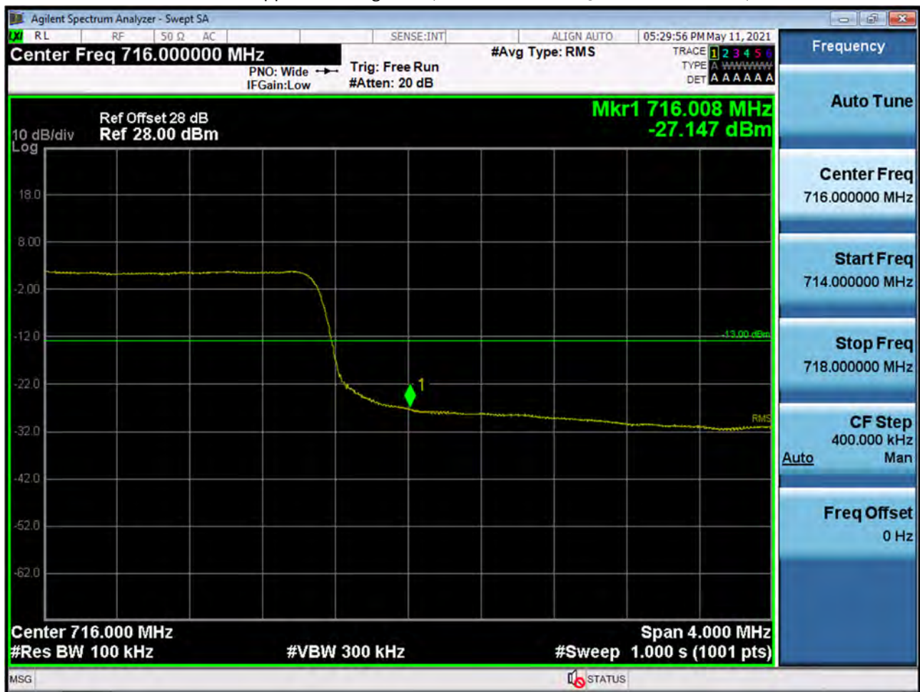
BAND 17. Upper Band Edge Plot (10M BW Ch.23800 QPSK_RB50_Offset 0)
