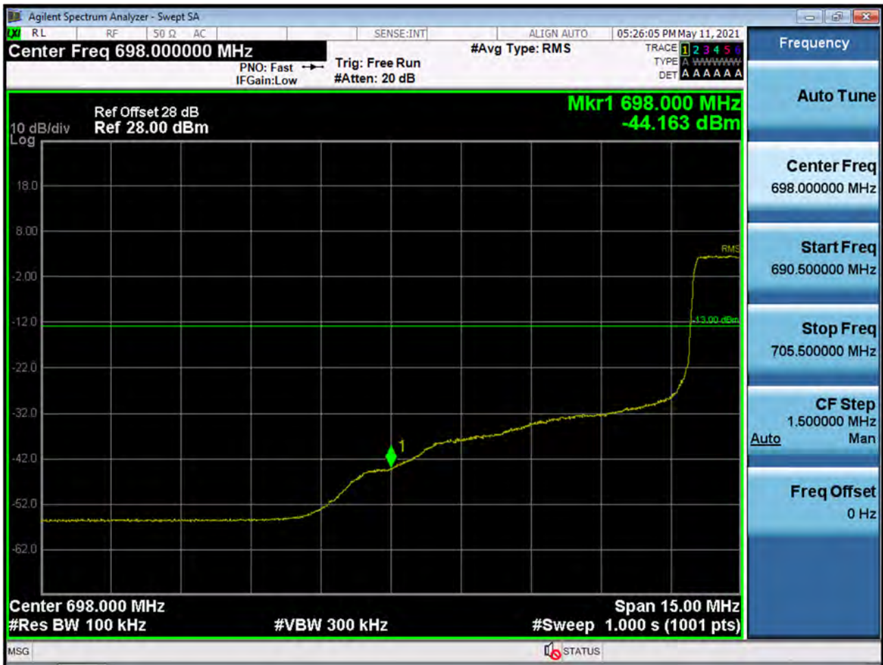
BAND 17. Lower Band Edge Plot (10M BW Ch.23780 QPSK_RB50_Offset 0)
