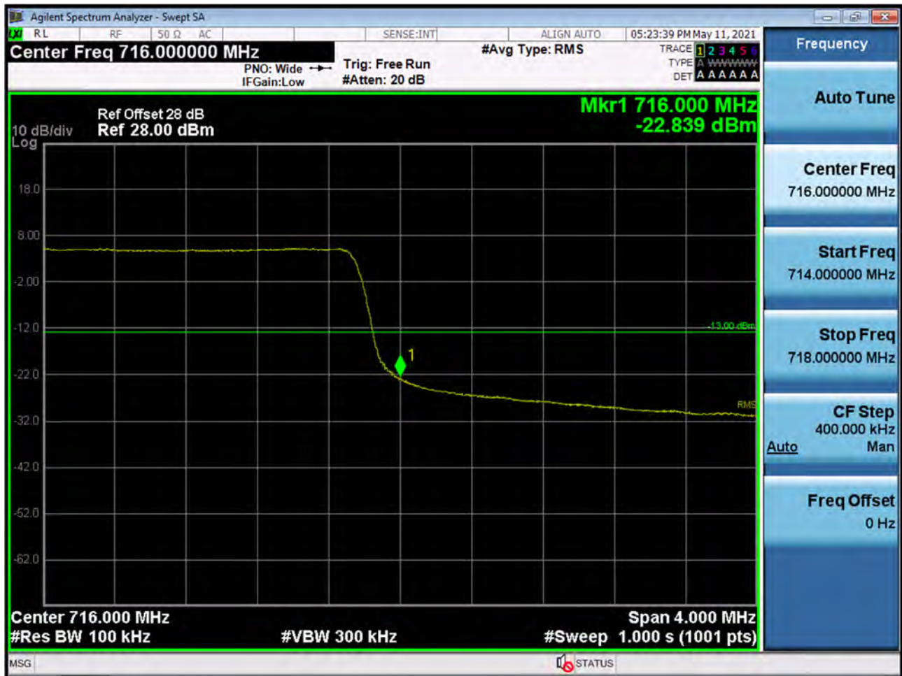
BAND 17. Upper Band Edge Plot (5M BW Ch.23825 QPSK_RB25_Offset 0)
