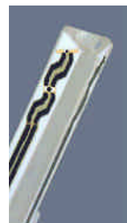
Figure 3.2 Probe Thick-Film Technique
