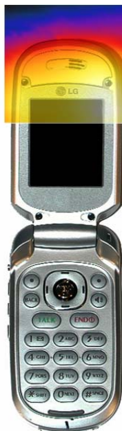
Figure 28 Sample H-field Scan Overlay
