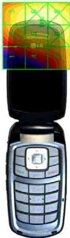
Figure 17-4 E-Field WD Scan overlay
