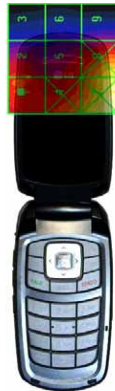
Figure 17-5 H-Field WD Scan overlay
