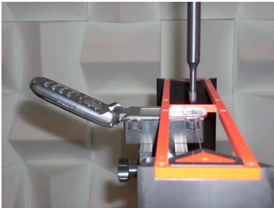
Figure 17-1 Ear Reference Point HAC Phantom Alignment
