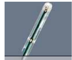
Figure 5-2 H-Field Free-space Probe
