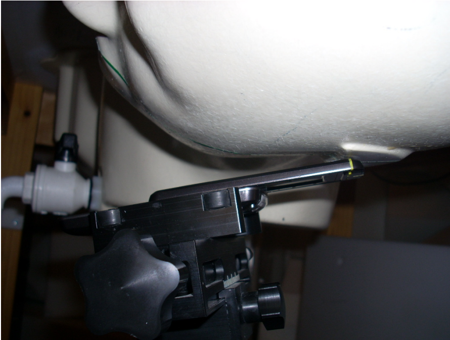
16. Left Head SAR, 15° Tilt, Slide Out
