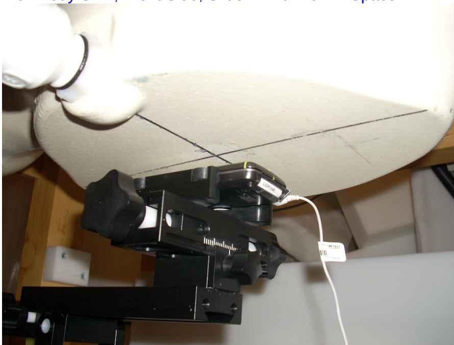
10. Body SAR, Front Side, Slide In with 20mm Space
