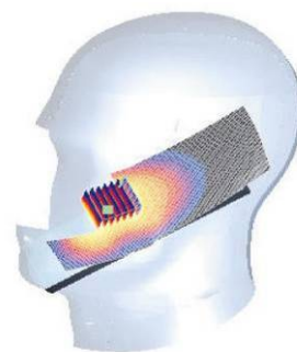
Figure 7-1 Sample SAR Area Scan
