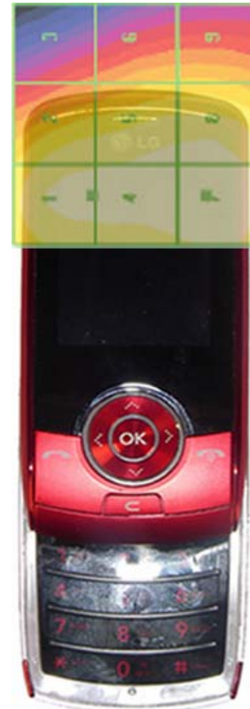
Figure 17-5 H-Field WD Scan overlay
