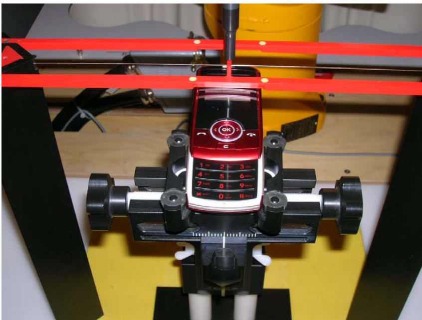
Figure 17-2 HAC Phantom Plane Alignment
