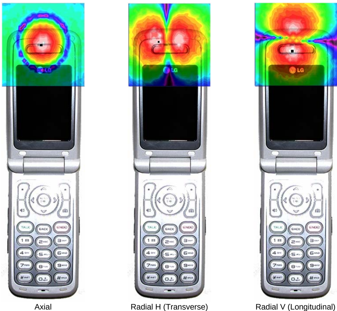
Figure 13-3 T-Coil Scan Overlay Magnetic Field Distributions
