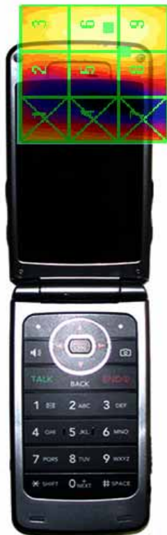
Figure 17-4 E-Field WD Scan overlay
