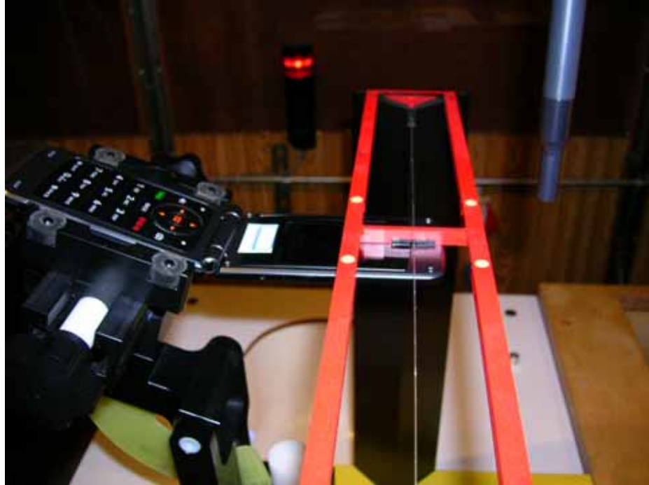
Figure 17-1 Ear Reference Point HAC Phantom Alignment
