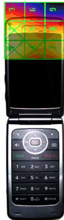
Figure 17-5 H-Field WD Scan overlay
